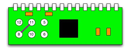
The number in each hole represents a Cool Muscle Pin #. 8 and 11 need to be connected by a jumper on the board or in the cabling.
